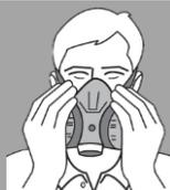
Negative pressure sealing test
