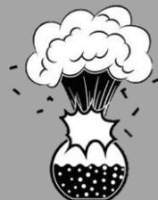
Cryogenic liquids must not be stored in closed containers, equipped with a sealing plug (or hermetically), nor in a thermos bottle. Indeed, if the container is closed tightly, the gas then can't escape; so there is risk of explosion.
